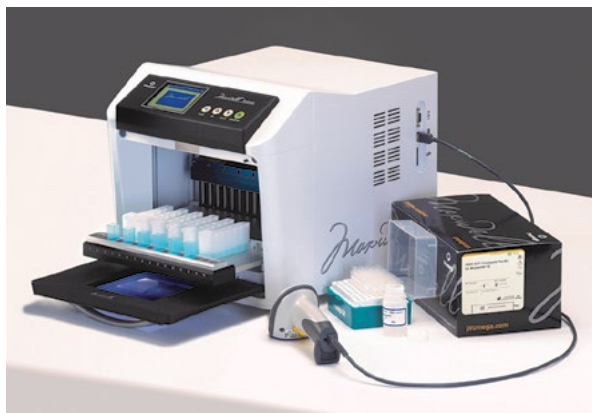
Maxwell ® 16 (left) and DNA IQ ™ Casework Pro Kit (right) are used by crime labs globally to isolate and purify DNA.
