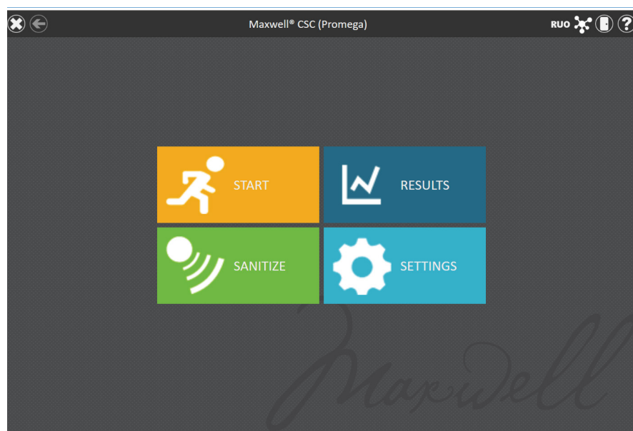
Figure 22. 'Home' screen. Selecting the Start button begins the process of running an extraction method on the Maxwell® CSC Instrument.
