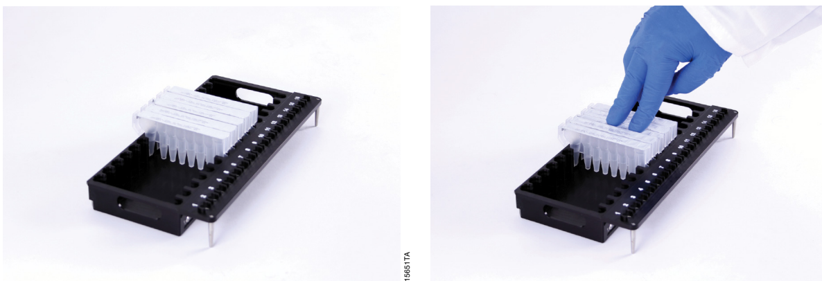
Figure 30. Placing the cartridges in the Deck Tray and pressing firmly to snap in place.
