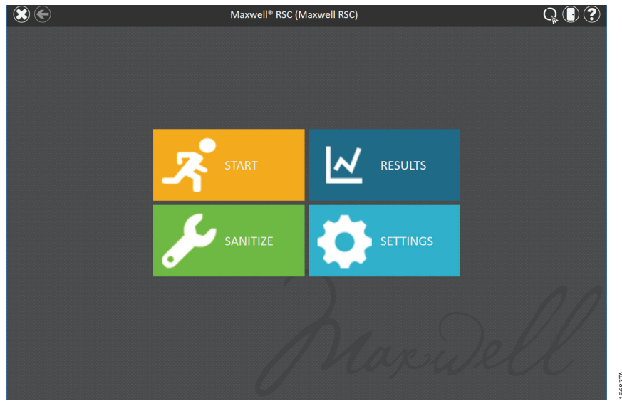
Figure 61. Maxwell® RSC 'Home' screen. Selecting Results opens the Maxwell® RSC 'Results' screen from which extraction reports from all method runs can be viewed.
