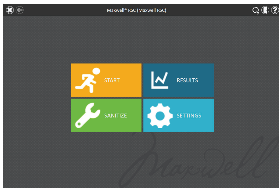
Figure 52. Maxwell® RSC ‘Home’ screen. When the Quantus™ Fluorometer is correctly connected to the Maxwell® RSC instrument, the “Q” logo is displayed in the upper right corner of the title bar.
