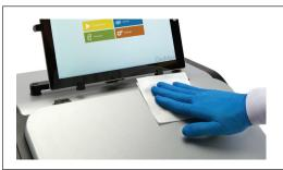
**3.** Use a soft clean cloth dampened with deionized water to periodically clean the exterior of the instrument.
